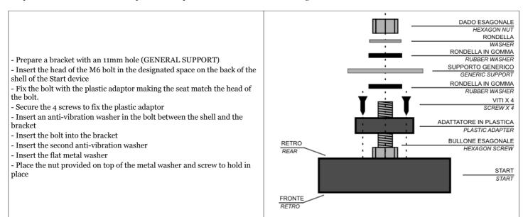
Please note: absence of anti-vibration washers or incorrect positioning of these could damage the device due to vibrations of the vehicle. This type of damage is not covered by the guarantee as it is not caused by a product defect but incorrect installation.
