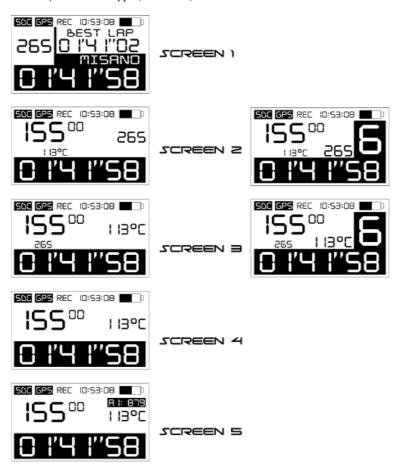
On screens 2 and 3, visualisation of the gear can be deactivated (image on the left) or activated (image on the right); follow the instructions in Chap. 11 for gear settings.
